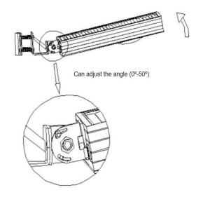
To place the light pole into the best spot with good day lighting. The light pole should be the length 4-6m, the thickness 2.0mm with material iron or steel, the diameter 50-90mm.
